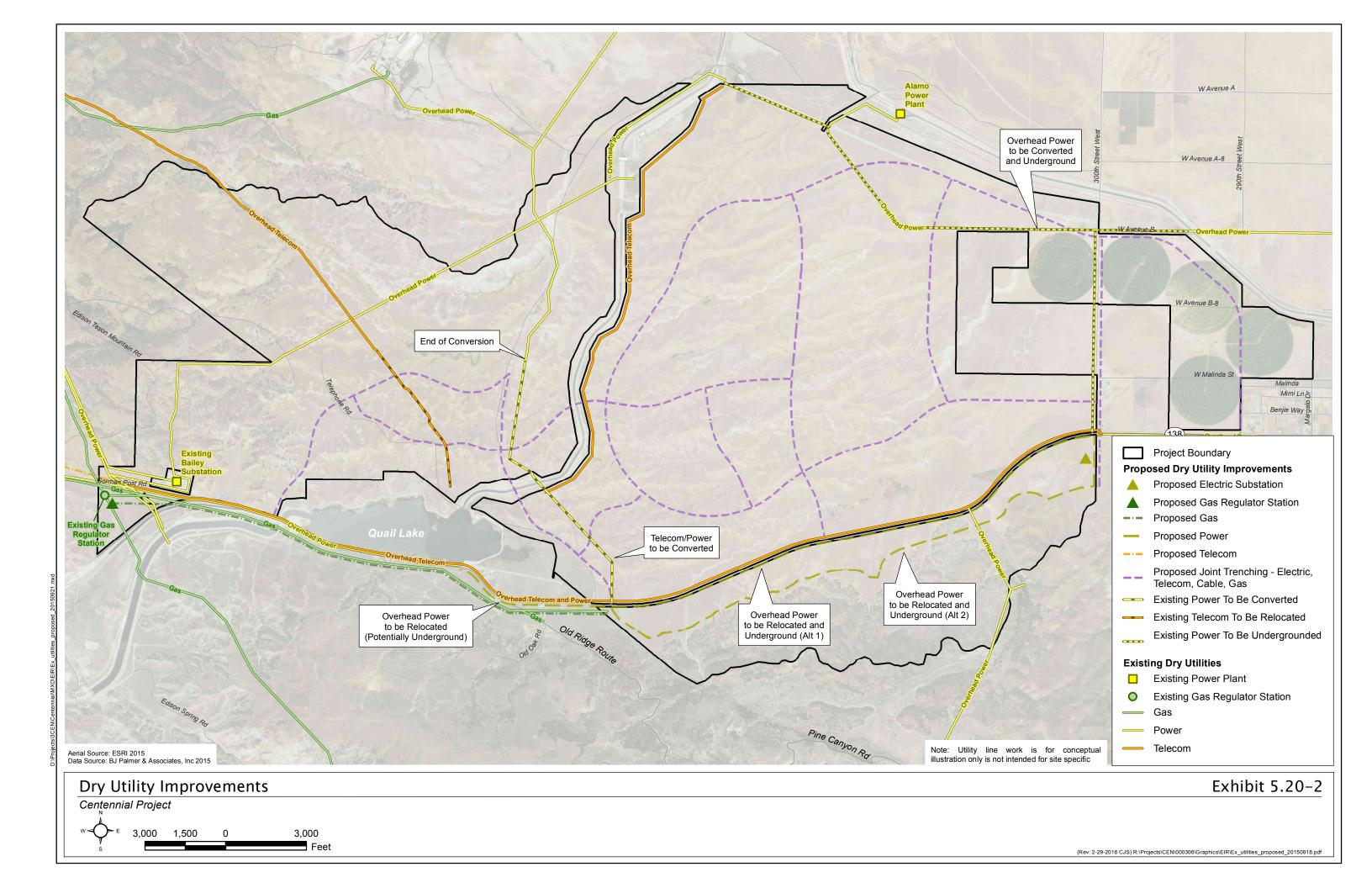
to the north of the Project site. Currently, approximately 300 dwelling units could be served by the existing overhead facilities associated with the Gorman Substation before a utility upgrade would be required (BJ Palmer 2015).
